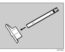
Temporarily fasten one long screw in the position, as shown. Turn the screw three to four times by hand.
