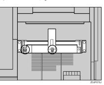
Fasten the right side of the connecting bracket using a long screw and the provided screwdriver. Also tighten the two screws temporarily tightened in step 13.
