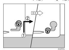
With the left corner of the mounting bracket in the position pointed by the arrow on the printer, fasten the left side of the mounting bracket using a long screw and the provided screwdriver. Also tighten the screw on the right side temporarily fastened in step **P**.
