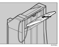
Fasten the finisher tray using a short screw and the provided screwdriver.
