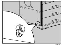
Insert the rail, assembled in step  $\overline{\mathbf{y}}$ , into the base area under the printer.
