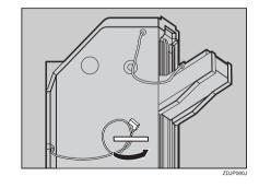
Connect the cable of the 2 tray finisher to the lower connector on the back of the printer.
