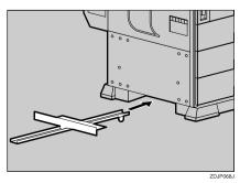
Hook the hole of the mounting bracket on the screw temporarily fastened in step 9.
