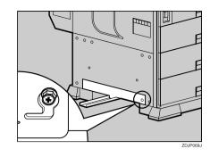
Holding the mounting bracket using both hands, move it in the direction of up (1) to the right (2).
