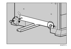
**13** Temporarily fasten the two long screws in the positions shown. Turn the screws three to four times by hand.
